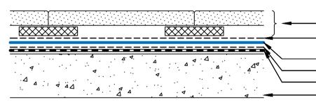
CONCRETE TILES ON BRICKS - OF EXTRUDED POLYSTYRENE OR SUPPORT PADS
